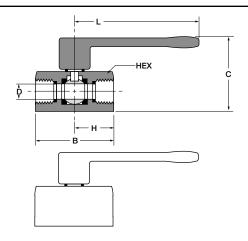
Male-Female Pipe Ends, Compact Handle, Mini Ball Valve MV608
