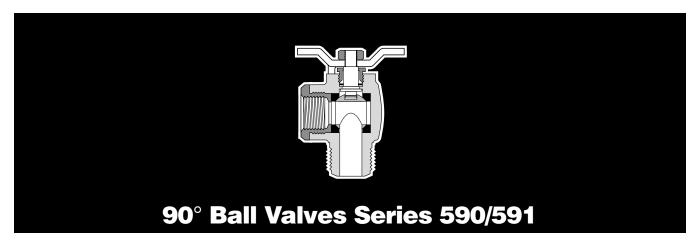
Parker's forged body valve provides extended service life and resists failure caused by severe temperature applications. Optimum flow design assures maximum system efficiency. Highly inert PTFE seats and seals provide resistance to chemical corrosion. Parker also provides a blow-out proof stem and chrome plated brass ball on all series 590/591 valves. Parker's 590/591 series valve bodies are machined from high quality CA377 forgings.
