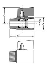
Female Pipe Ends, Compact Handle, Mini Ball Valve MV609
