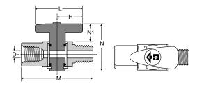
Female Pipe to Female Pipe Plug Valve PV609
