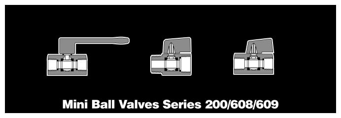
The Parker Mini-Valve is to be used in confined and hard to reach applications. The Brass extruded body allows for extended service life and is chrome plated as standard. Features of the MV608/609 valves include blowout proof stem, hard chrome plate ball, PTFE seats, viton stem seals, and standard yellow handle. MV200 valve features a black lever handle. This economical ball valve is available in 1/8",1/4", 3/8" and 1/2" sizes.
