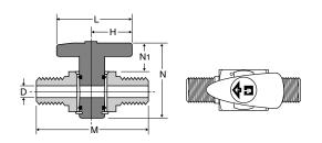
Female Pipe to Male Pipe Plug Valve PV608
