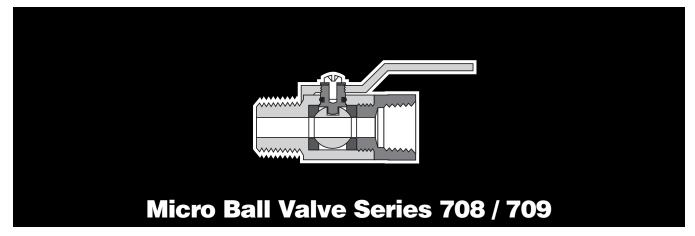
The Parker Micro-Valve is designed to be used in confined and hard to reach applications. This miniature 2 way valve has a barstock body for extended service life and is offered with either male / female or female / female pipe ends. Features of the MV708 / 709 valves include chrome plate ball, PTFE seats, nitrile stem seal and a low profile chrome plated steel handle.
