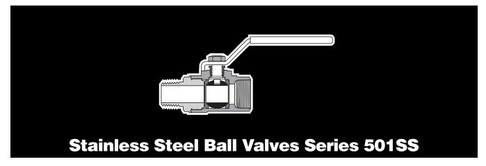
Parker's Cast Body is manufactured from CF-8M Stainless Steel, the cast equivalent of 316 Stainless Steel. They are ideal for corrosive environments such as chemical plants and refineries. The full flow design assures maximum operating efficiency. The reinforced PTFE seats and seals, coupled with the 316 Stainless Ball and blow-out proof stem, result in the utmost reliability. This ball valve is available in 1/4", 3/8", 1/2", 3/4" and 1" female pipe sizes.
