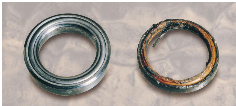
Fig.7 Before and after. This polypak rod seal has been damaged by water, a common contaminant in mineral oil systems.
