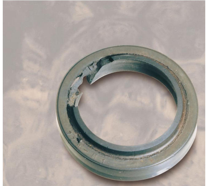
Fig.9 The rod wiper may extrude (top) but the primary rod seal looks perfect (right), so no leakage occurs when the cylinder is hydrostatically tested.
