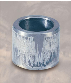
Fig.4 Particle contamination has scored the surface of this cushion bush, resulting in loss of cushioning effect.
