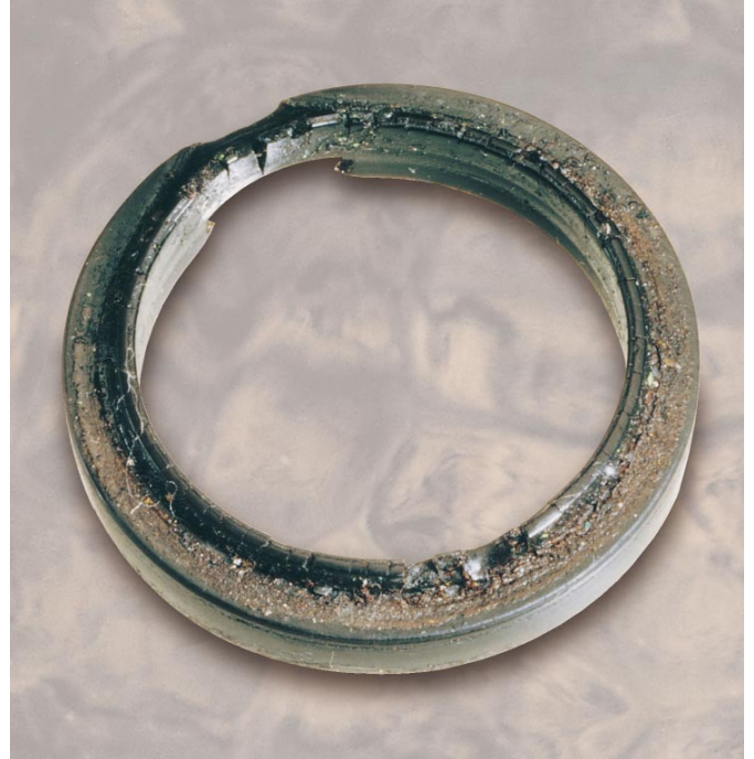
Fig.6 The cracked outer sealing lip of this wiper seal shows damage caused by heat.
